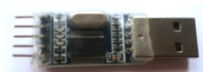
**Figura 4.1:** Conversor USB a TTL
