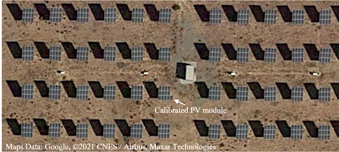
Fig. 3.1. The photovoltaic plant under study in Granada, Spain, has a datasheet nominal power of 109.44 kW. Top: Photo taken at ground level. Bottom: Satellite Image (Latitude: 37.287, Longitude: -3.057).
