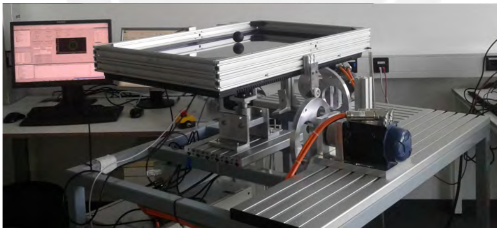
Figure 3.5: Ball and plate system implemented by the Control Engineering Group of TU Ilmenau [3].
