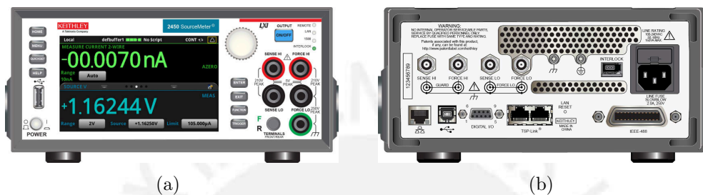
Figura 3.11: Keithley 2450 (a) Frontal (b) Posterior.
