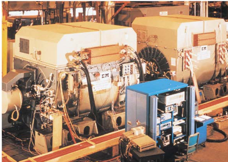
Figures 58 Back to back test of 2-14200 HP 3200 RPM 2 pole synchronous motors for VFD application. The shaft extensions are coupled together, and with their respective VFD's one operates as a motor and the other operates as a generator, achieving essentially full load operation of each machine. In this type of test the local utility must only make up the losses of the machines and VFD's.
