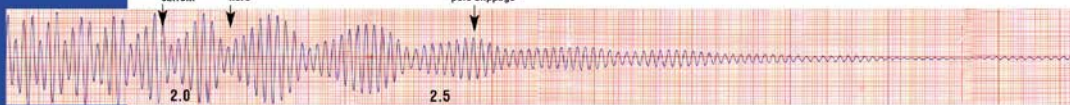
Figure 28b Stator Current. Rotor pulls into synchronism with minimum stator current. (Note: Pulsations of current after synchronism are oscillations due to very large flywheel effect of the load.)
