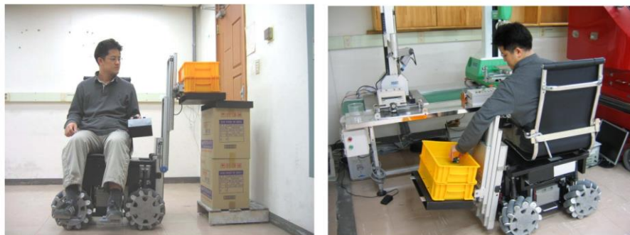
Fig. 1.6. Omnidirectional vehicle for disabled workers. Image taken from Kang et al.
