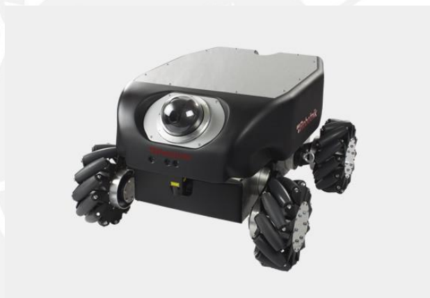
Fig. 1.5. SUMMIT-X from Robotnik for automated omnidirectional motion. Image taken from www.robotnik.eu
