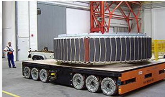
Fig. 1.5. Kuka's KMP omniMove, design for heavy-duty-transport. Image taken from www.kuka-robotics.com
