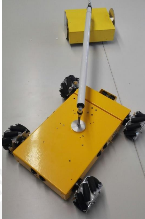
Fig. 4.12. The telescopic pole, which connects robot and trailer, allow the connecting distance to vary between the two bodies of the system
