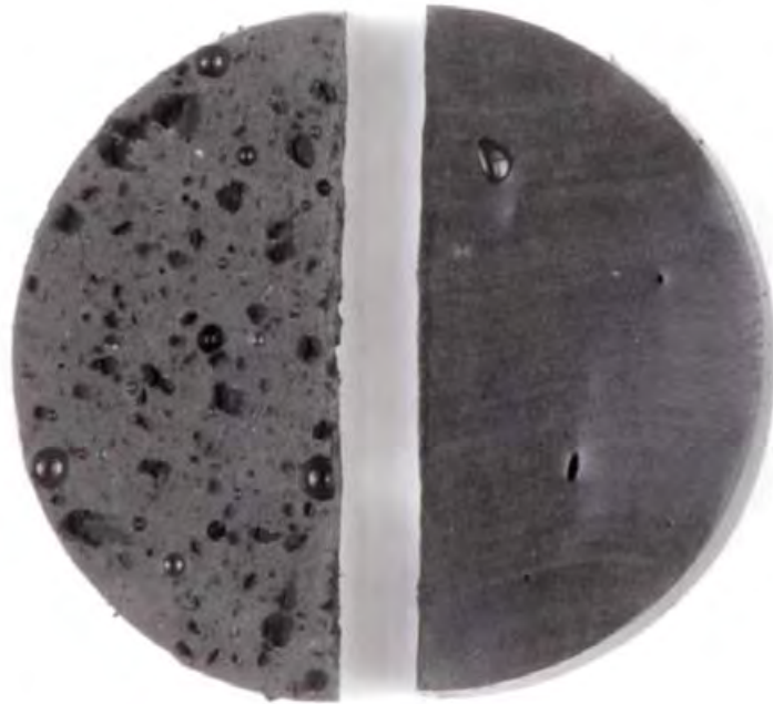
Figure 2.2: Difference between a sample with unsieved graphite (left) and sieved graphite (right). Photo made by Tobias Kaufhold.
