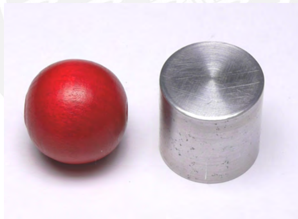
Figure 2.25: Objects inserted to the samples on the experiments, on the left a ball, on the right a cylinder, both with 20mm diameter.
