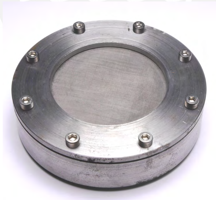
Figure 2.1: Set up for sieving graphite with the 25 microns size mesh.
