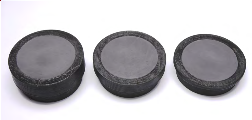
Figure 2.24: Samples used on field-induced plasticity tests. From left to right 20mm, 15mm and 10mm in height and 40mm diameter for all samples.
