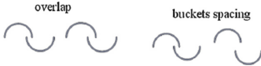
Figura 18: Descripción gráfica del overlap ratio y el buckets spacing (Akwa, Vielmo, & Petry, 2012)
