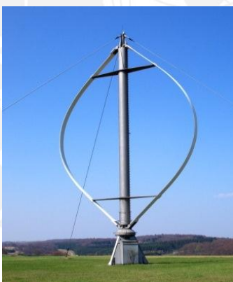
Figura 1: Aerogenerador de eje vertical Darrieus Eggbeater;
