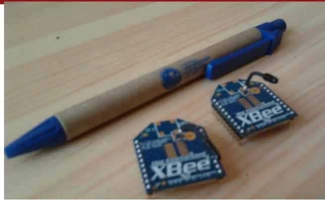
Figura 6: Módulos RF XBEE Series 2 International a utilizar
