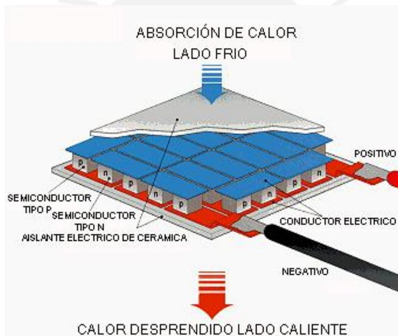
**Figura 2.3: Celda peltier**
