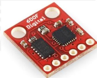
Fig. 3.2 – 5: Sensor Inercial
