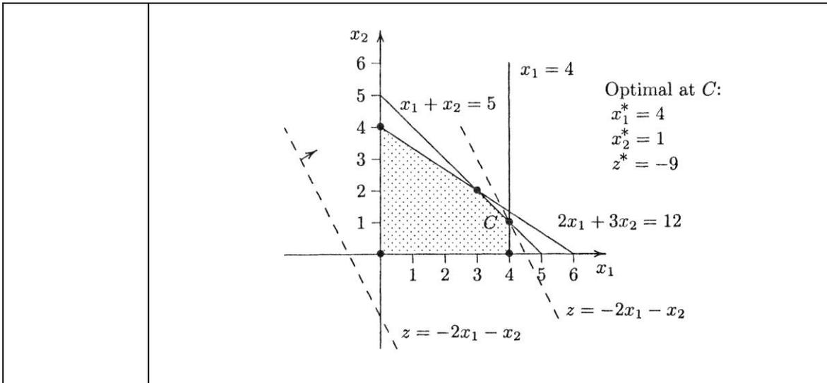
Figure 2-1: Graphical Solution of a Two-Variable LP
