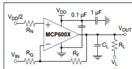
**FIGURE 1-2:** AC and DC Test Circuit for Most Inverting Gain Conditions.
