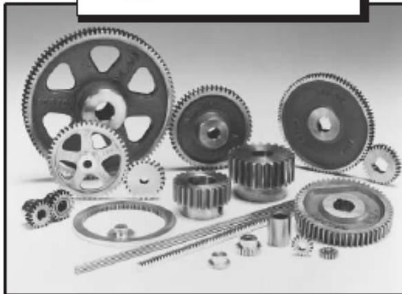
*Boston spur gears are designed to transmit motion and power between parallel shafts. Configurations include spur, rack, pinion wire, stem pinions and internal gears; most with a selection of bores, keyways and set screws. Fine-pitch gears are available in plastic, brass, stainless steel and steel. Heavier pitch spurs are available in steel and cast iron. Styles include plain, web, web with lightening holes or spoked. Change gears have consecutive numbers of teeth for a variety of ratios.*
