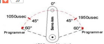
This servo can be configured to operate 180° by using any of the following servo programmers:
