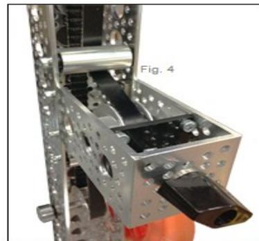
Shown incorporated into a belt tensing system - the Idler Shaft A fits perfectly inside [channel](#).
