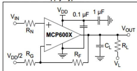
**FIGURE 1-1:** AC and DC Test Circuit for Most Non-Inverting Gain Conditions.
