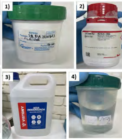
Figure 10 Supplies: 1)Yungay Potato Starch, 2) Barium Titanate Oxide (BTO) 3) Distilled Water 200mL 4) Glycerol (Plasticizer) 4gr0
