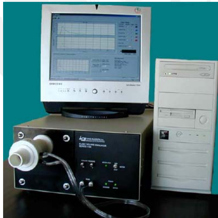
Figura B-3: Series 1120 Flow / Volume Simulator.
