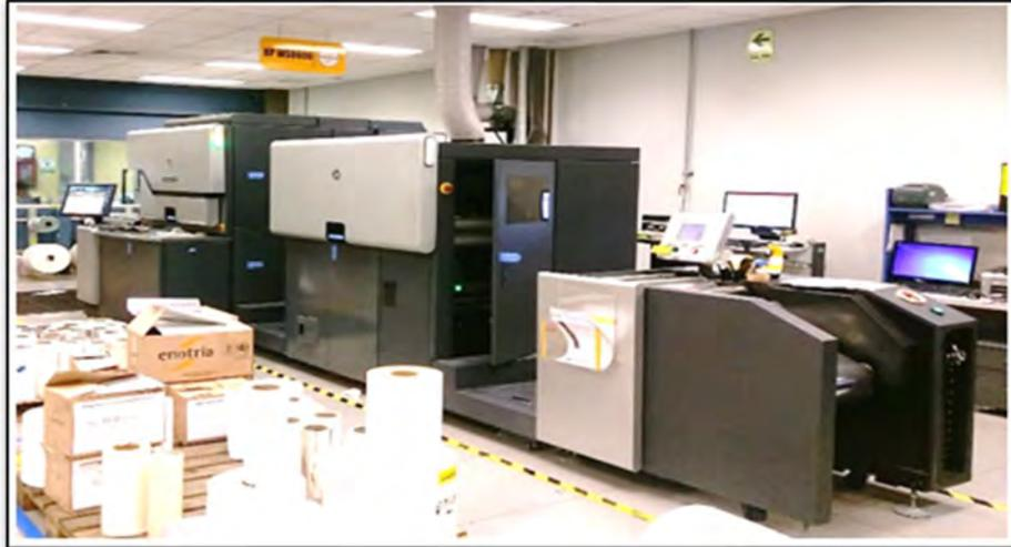
Figura 21: Máquina HP Indigo WS6600
