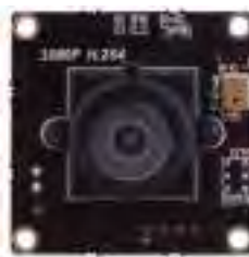
Figura 5.4: Low-light HD USB camera (Fuente: www.bluerobotics.com ).
