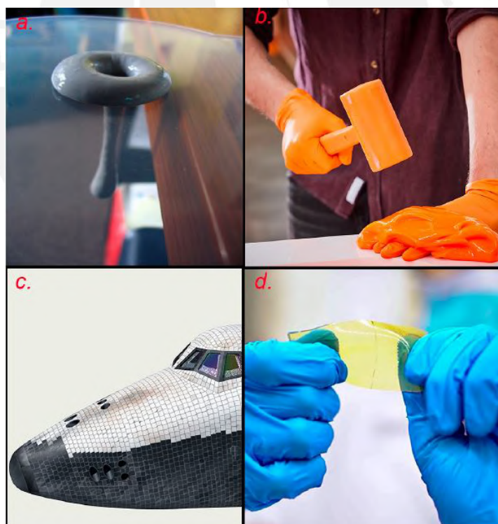
Figure 2.8.: Applications of PBS: (a) As rheological liquids; (b) for the manufacture of protection against mechanical damage; (c) as fire-resistant ceramics; (d) as self-healing material [8]
