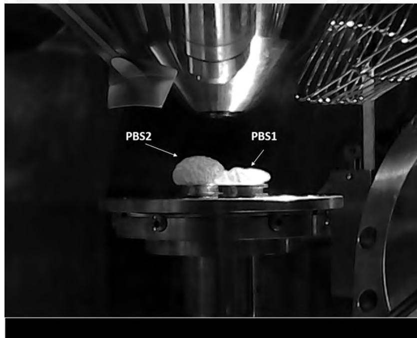
Figure 5.6.: PBS1 and PBS2 samples during the vacuum process
