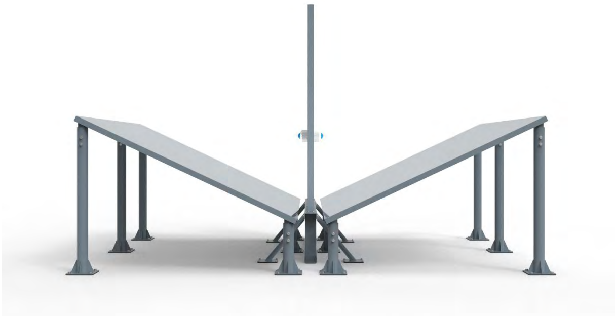
Fig. 14 South (Frontal) view of the VBF, reflectors and pyranometers.
