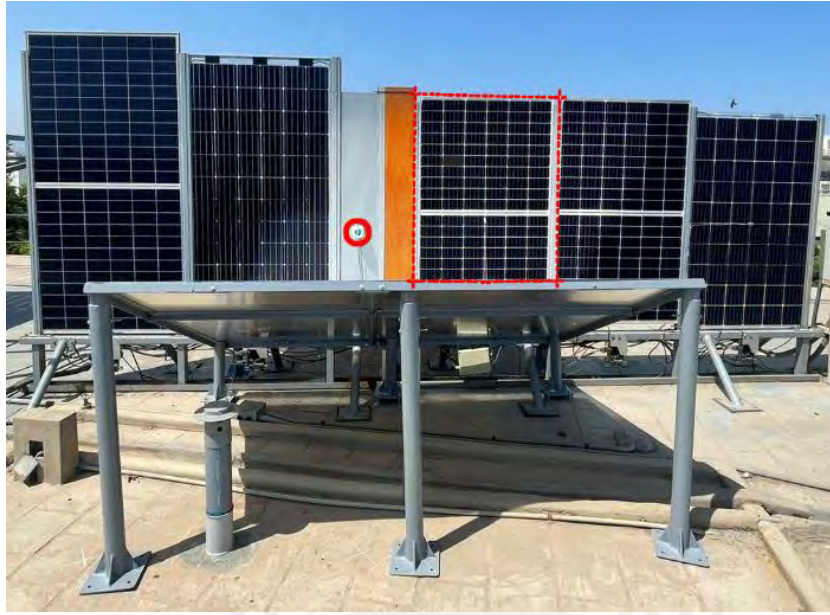
Fig. 22 East (lateral) view of the arrangement. Circled in red is the module used for testing as well as the pyranometer.
