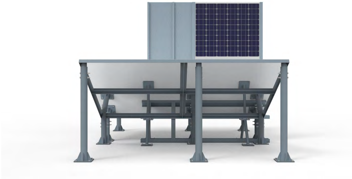
Fig. 13 East (Lateral) view of the VBF, reflectors and pyranometers.
