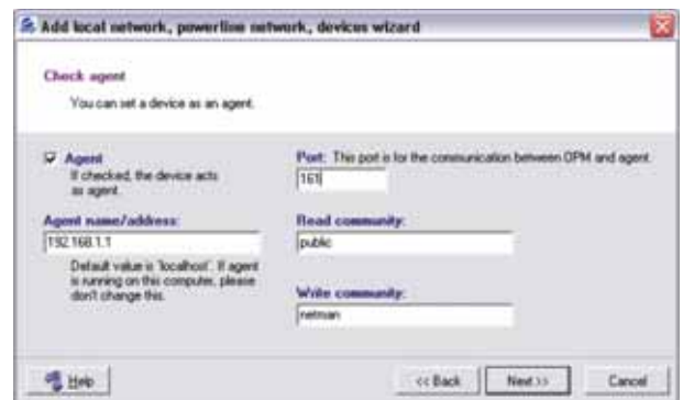
Adding Powerline Device - Powerline Agent Settings
