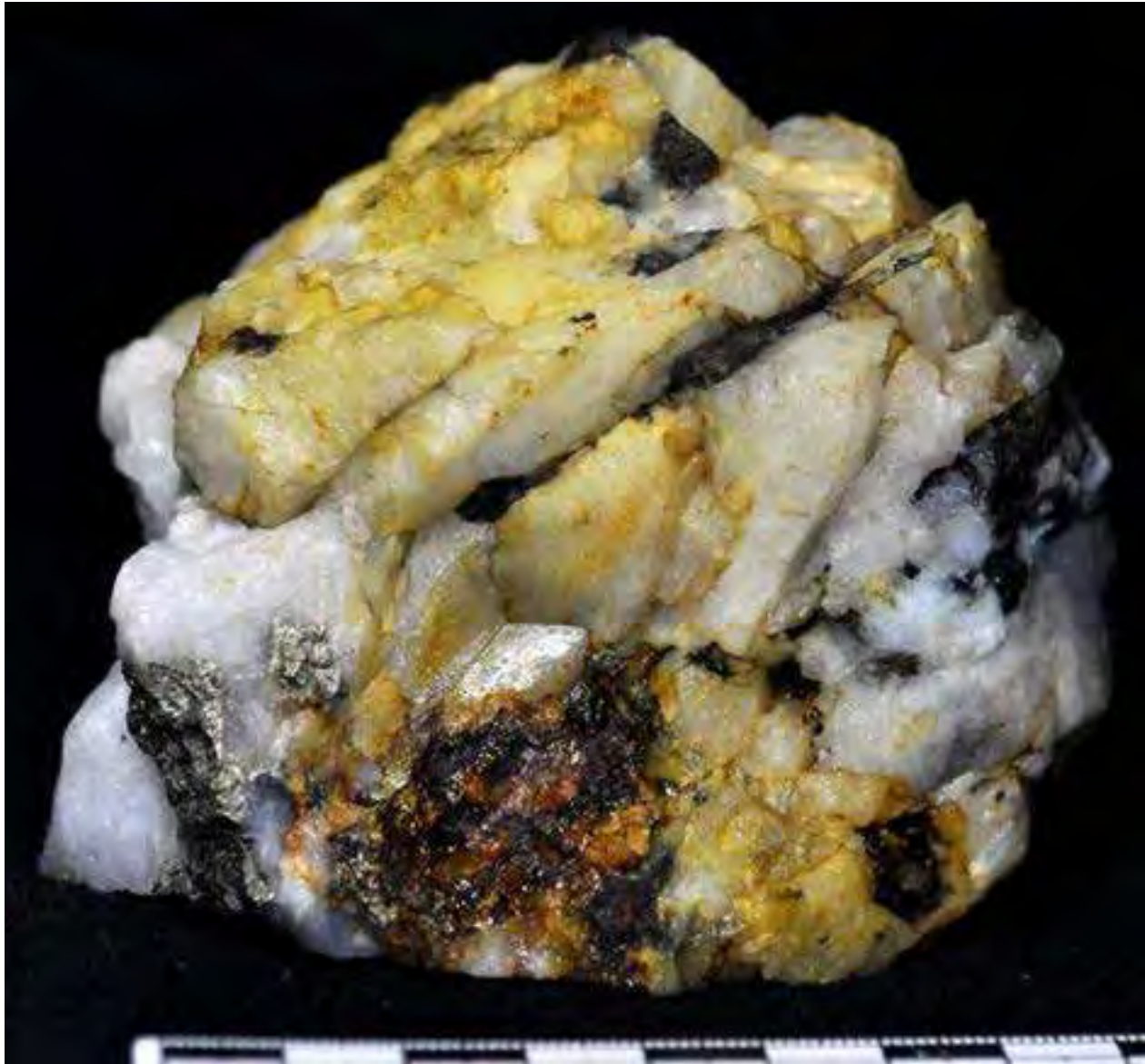
Mineralized vein composed largely of quartz, pyrite and Fe-rich carbonates. Quartz is milky and forms mm- to cm-sized subhedral to euhedral crystals. Pyrite and Fe-rich carbonates appear lining fractures and interstitial space between the quartz crystals. Pyrite forms mm- to cm-sized aggregates of mm-sized subhedral to euhedral grains.
