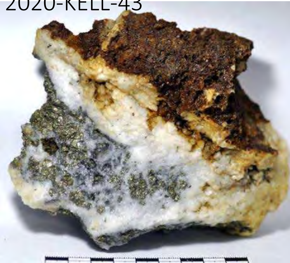
Mineralized vein composed mostly of quartz, pyrite, and lesser amounts of arsenopyrite. Massive milky quartz is locally overgrown by subhedral semi-translucent quartz crystals up to 0.5 cm long. Pyrite appear forming individual crystals and centimetric aggregates within secondary porosity in quartz. Arsenopyrite is intergrown with the quartz and forms millimetric aggregates of subhedral crystals.
