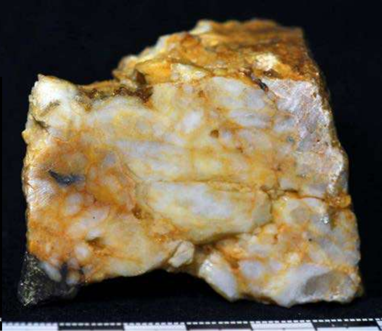
Mineralized quartz-cassiterite-Fe-rich carbonate vein. Euhedral-subhedral semi-translucent quartz crystals are up to 1.5 cm in length. Iron-rich carbonates form mm-sized brown, platy crystals that form aggregates on top of vein quartz. Pyrite forms millimetric aggregates of <1mm crystals.
