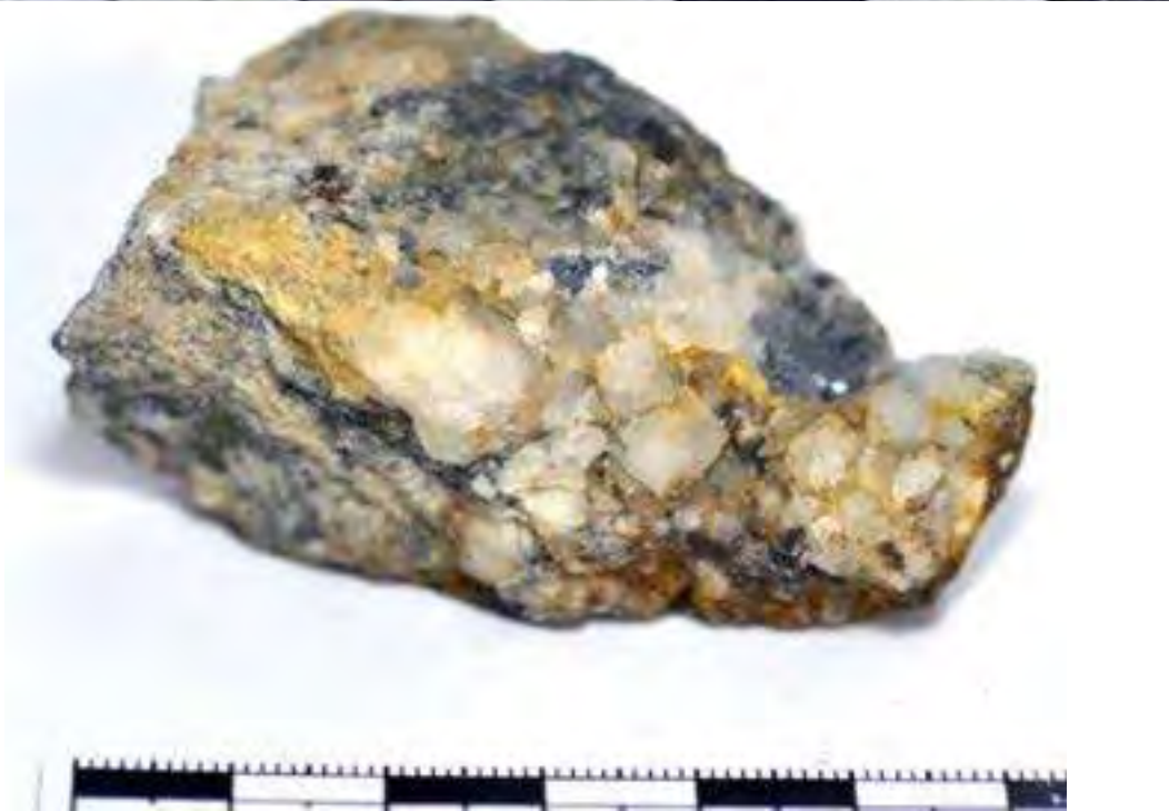
Quartz- and galena-rich vein. Quartz forms euhedral-subhedral translucent crystals up to 1 cm long. Black crystals (<1mm) (cassiterite?) appear scattered in the quartz and galena.
