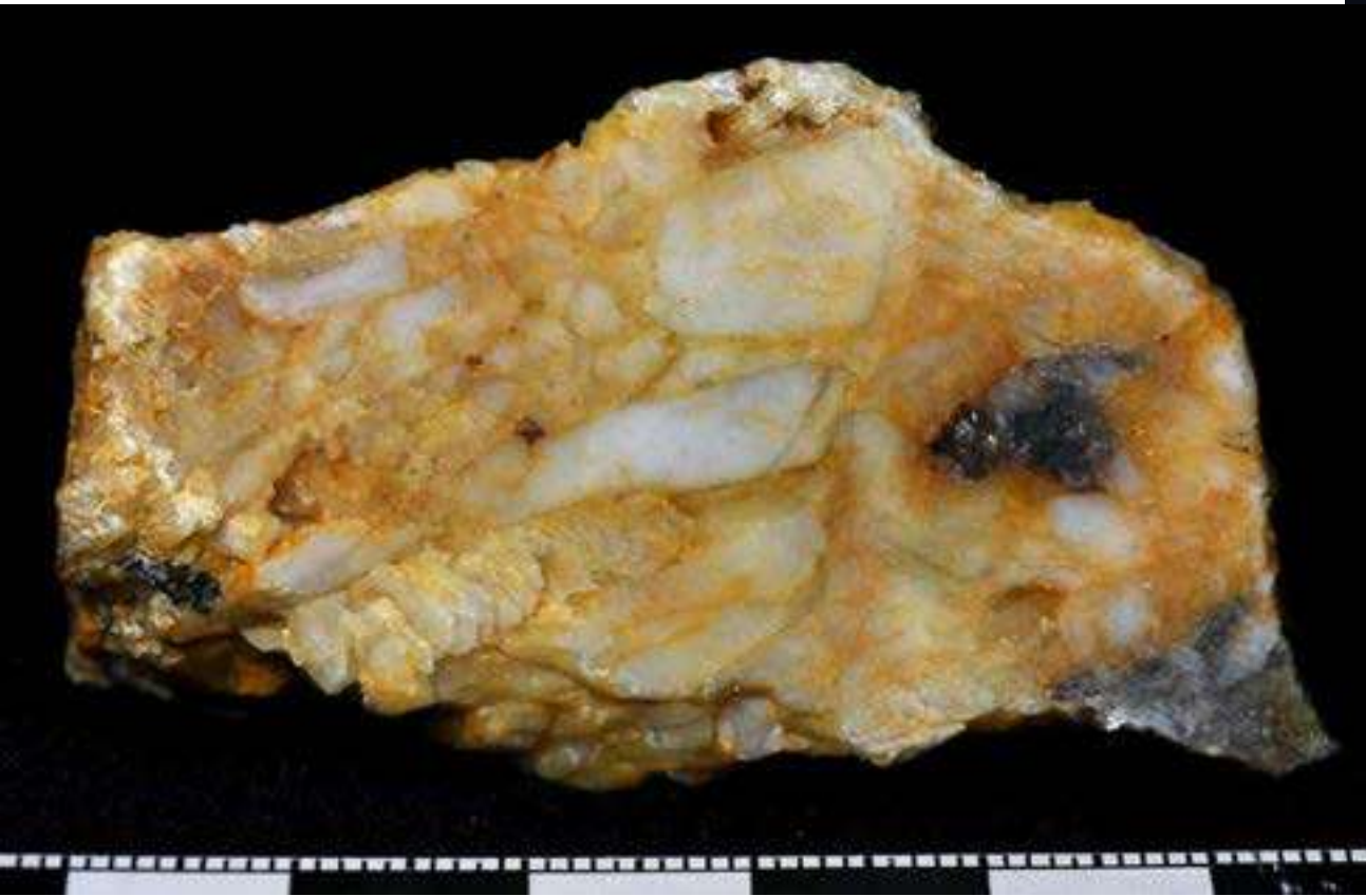
Mineralized quartz-cassiterite-Fe-rich carbonate vein. Euhedral-subhedral semi-translucent quartz crystals are up to 1.5 cm in length. Iron-rich carbonates form mm-sized brown, platy crystals that form aggregates on top of vein quartz. Pyrite forms millimetric aggregates of <1mm crystals.
