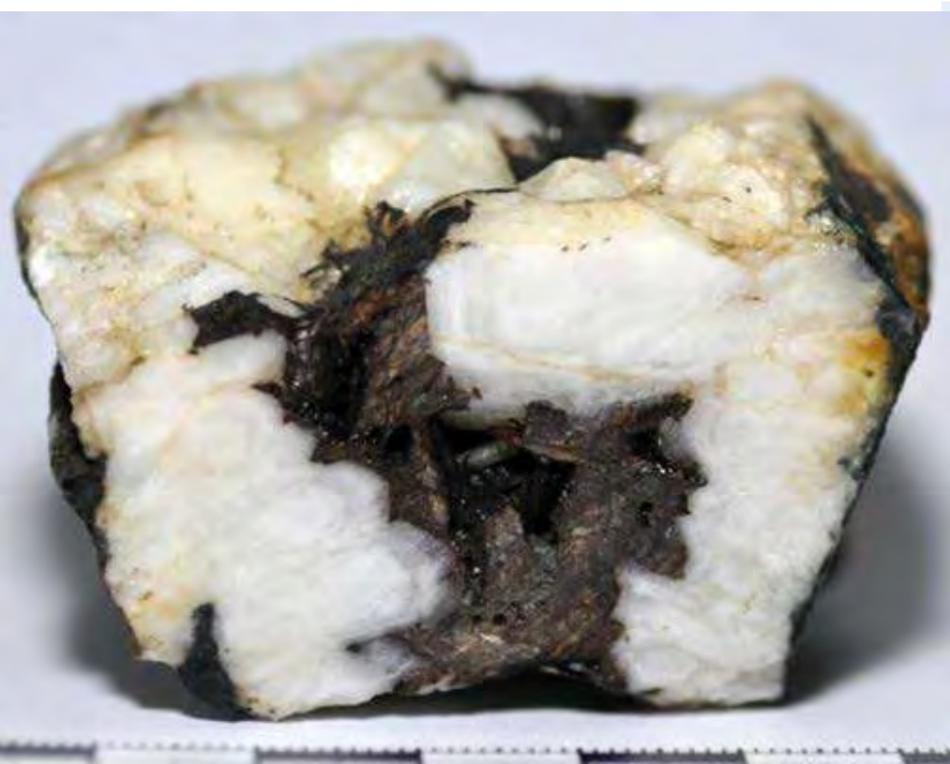
Mineralized quartz-carbonate-sulfide vein. From the contact with the host rock to the core of the vein, there is a gradation from euhedral to subhedral translucent quartz crystals up to 2 cm long depicting comb textures to Fe-rich carbonates. Quartz crystals show well-defined growth. Iron-rich carbonates form dark brown (partially oxidized), mm-sized, lens-shaped crystals. Pyrite and chalcopyrite are scarce and appear forming aggregates <0.5 cm intergrown with carbonates in the central suture of the vein.
