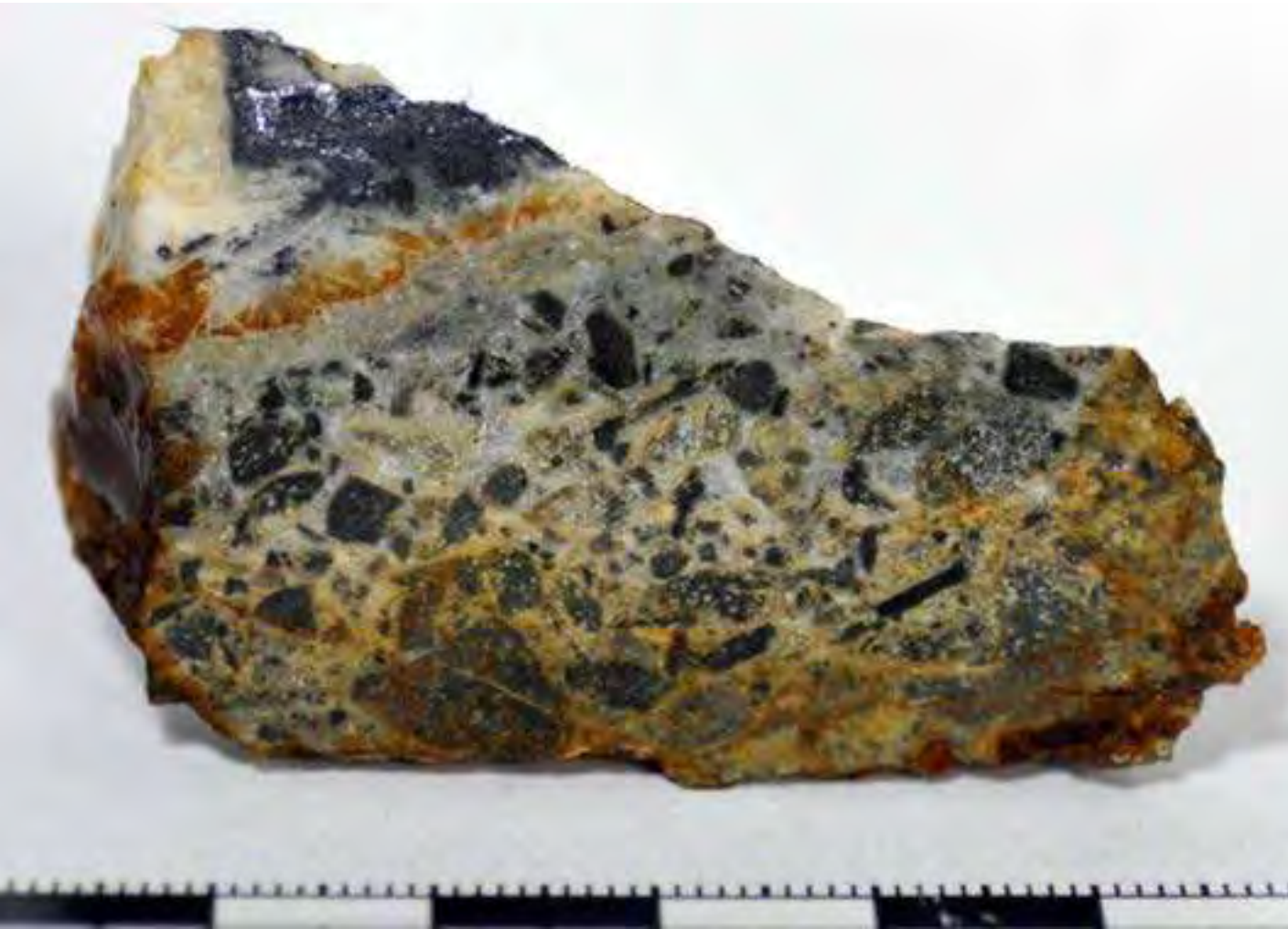
Mineralized hydrothermal breccia. Angular to sub-angular rock clasts up to 1 cm long, presumably from the hosting Catavi Fm., are cemented by semi-massive milky quartz. Some rock clasts have a porphyritic texture with white phenocrysts (<1mm), probably quartz or feldspars. The breccia is cut by a quartz-galena vein. Vein quartz crystals (1mm) are subhedral and translucent.
