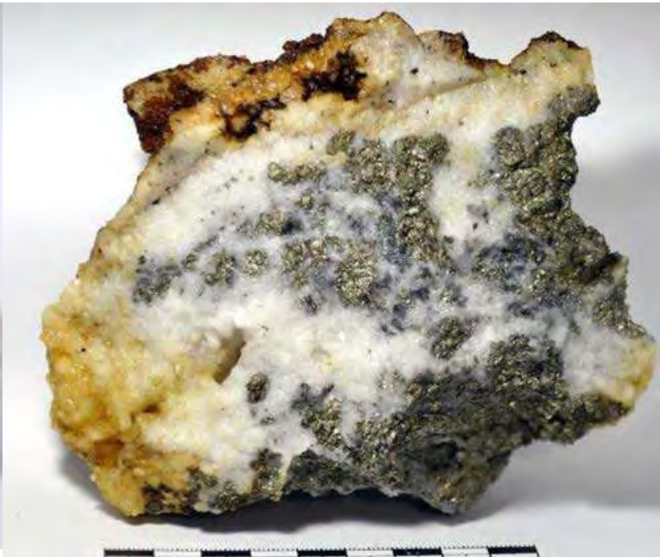
Mineralized vein composed mostly of quartz, pyrite, and lesser amounts of arsenopyrite. Massive milky quartz is locally overgrown by subhedral semi-translucent quartz crystals up to 0.5 cm long. Pyrite appear forming individual crystals and centimetric aggregates within secondary porosity in quartz. Arsenopyrite is intergrown with the quartz and forms millimetric aggregates of subhedral crystals.
