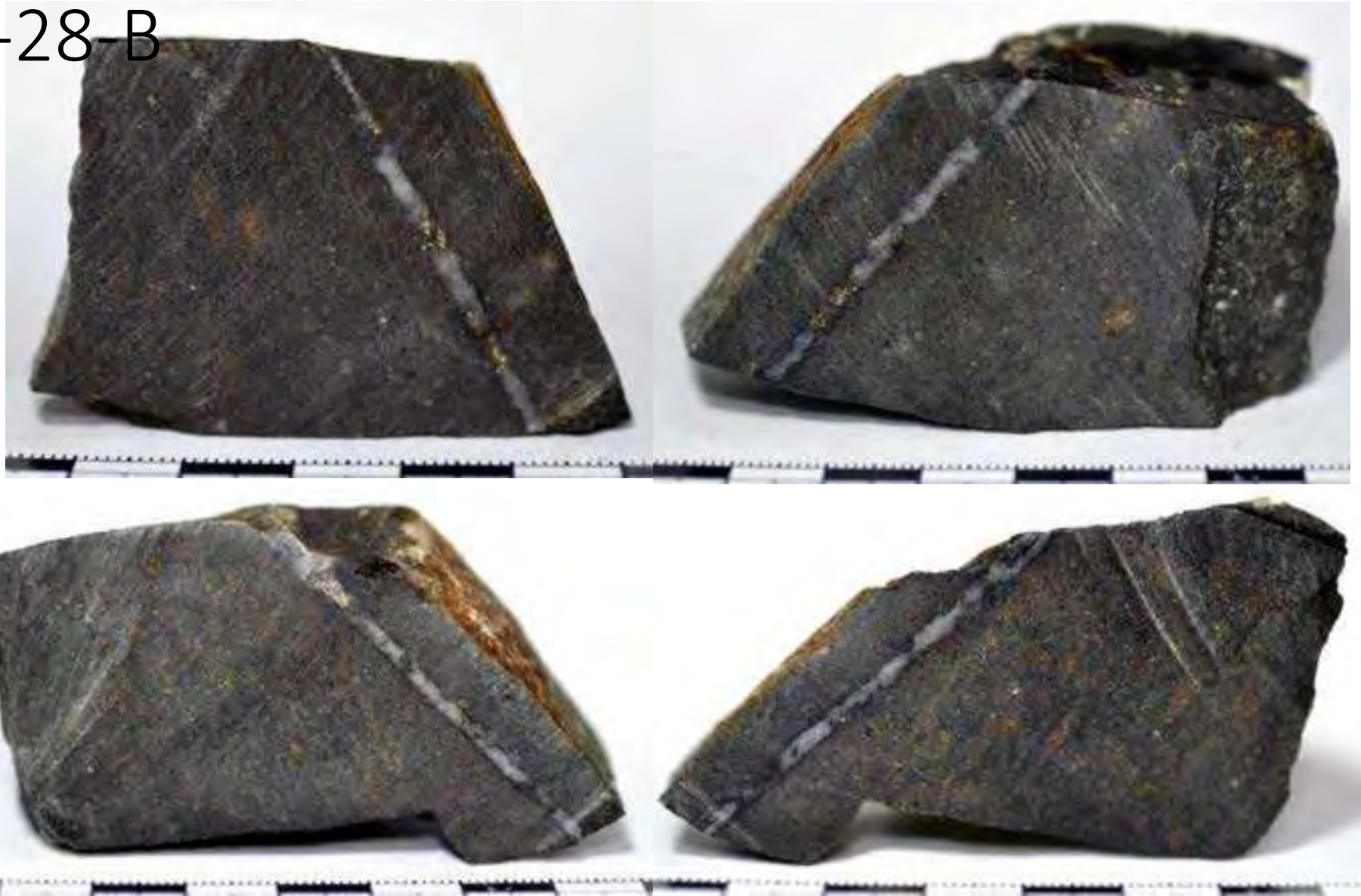
Quartz-tourmaline veinlets hosted by Catavi Fm. quartzites. Veinlets are up to 2 mm wide and are mostly composed of milky quartz and dark rims of tourmaline (<1mm wide). Oxidized pyrite is scarce and appears forming aggregates <4 mm across along with vein quartz.
