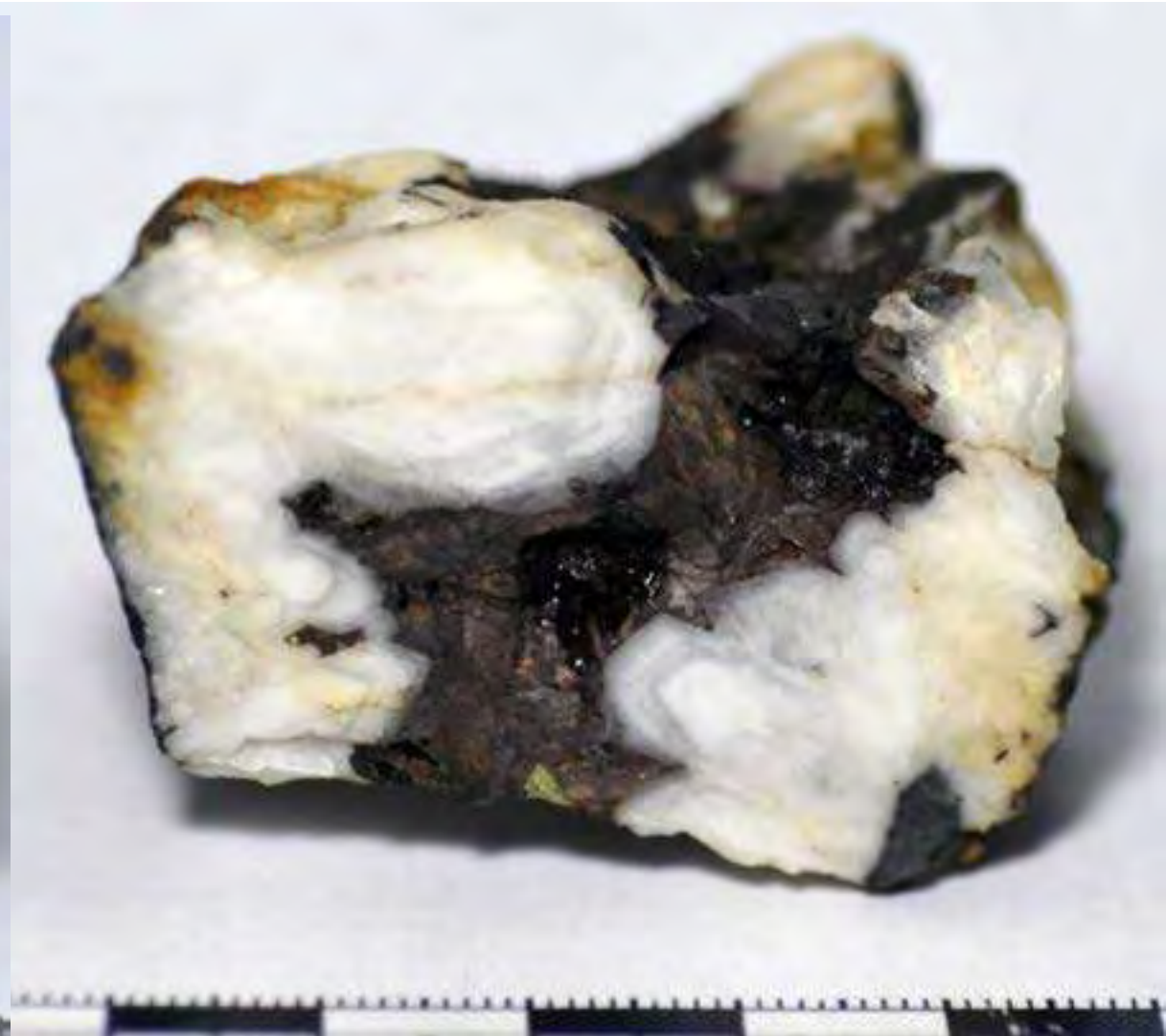
Mineralized quartz-carbonate-sulfide vein. From the contact with the host rock to the core of the vein, there is a gradation from euhedral to subhedral translucent quartz crystals up to 2 cm long depicting comb textures to Fe-rich carbonates. Quartz crystals show well-defined growth. Iron-rich carbonates form dark brown (partially oxidized), mm-sized, lens-shaped crystals. Pyrite and chalcopyrite are scarce and appear forming aggregates <0.5 cm intergrown with carbonates in the central suture of the vein.
