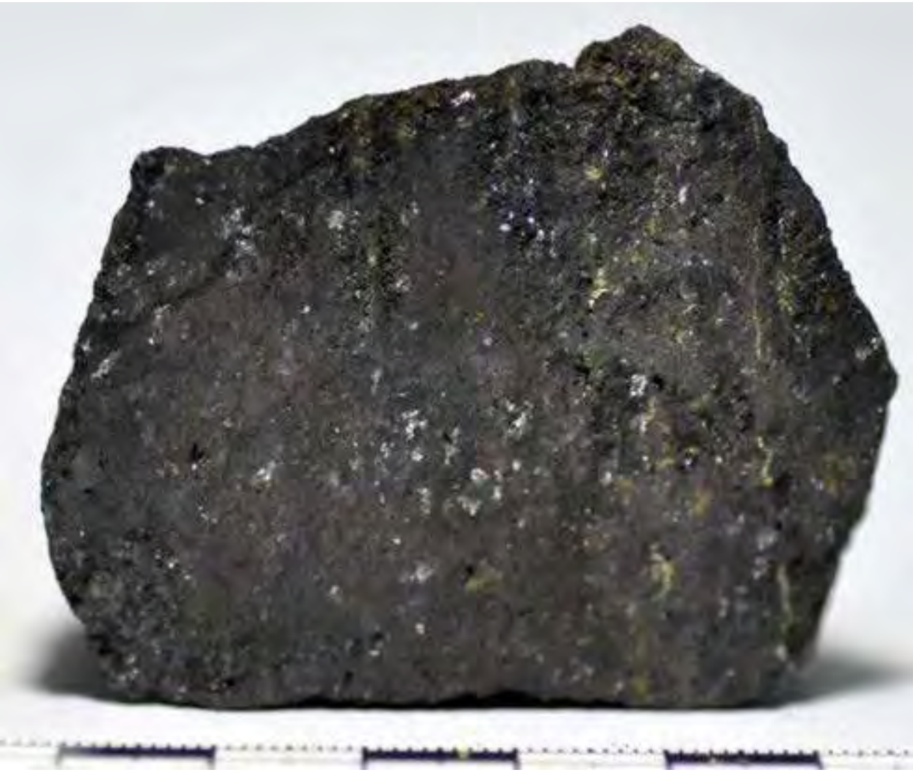
Black massive sphalerite ( var. marmatite) with lesser proportions of pyrite \pm chalcopyrite. The sample is composed in its great majority by black massive sphalerite although individual sphalerite subhedral millimetric grains are also observed. Subhedral-anhedral pyrite \pm chalcopyrite crystals appear forming mm-sized aggregates or thin veinlets across the sphalerite.
