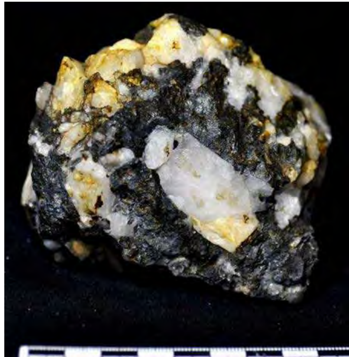
Mineralized vein composed largely of quartz, pyrite and Fe-rich carbonates. Quartz is milky and forms mm- to cm-sized subhedral to euhedral crystals. Pyrite and Fe-rich carbonates appear lining fractures and interstitial space between the quartz crystals. Pyrite forms mm- to cm-sized aggregates of mm-sized subhedral to euhedral grains.
