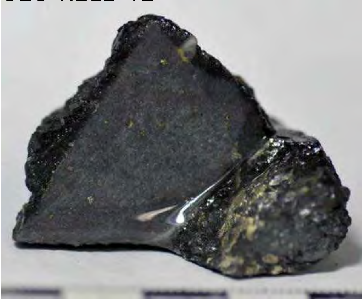
Mineralized vein composed of sphalerite, pyrite, milky massive quartz, and siderite. Sphalerite is massive and dark grey-black in color ( var. marmatite ). Pyrite forms millimetric- centimetric aggregates of subhedral-euhedral millimetric crystals and is intergrown with mm-sized subhedral platy siderite crystals. Veinlets of siderite-pyrite cut across sphalerite and milky quartz.
