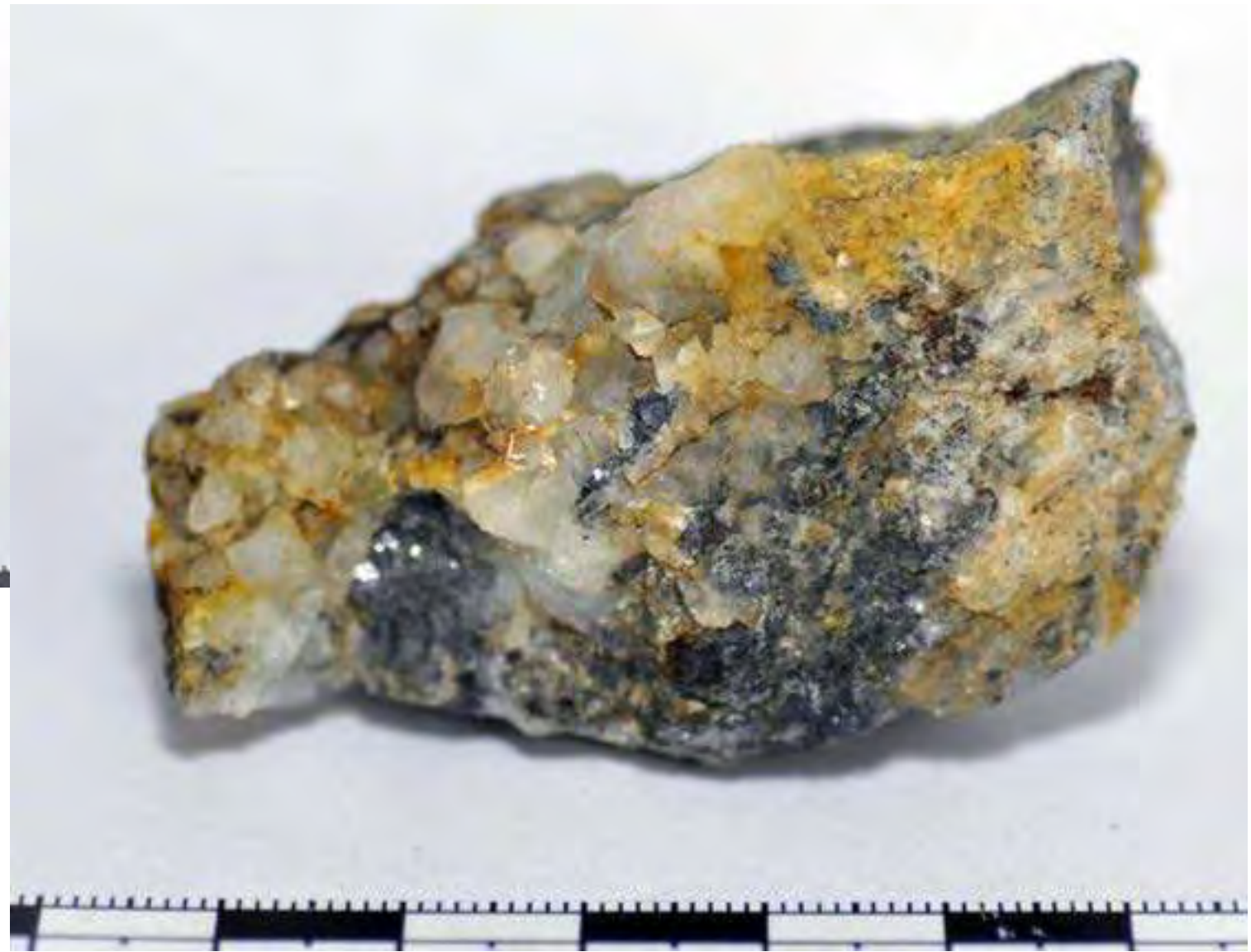
Quartz- and galena-rich vein. Quartz forms euhedral-subhedral translucent crystals up to 1 cm long. Black crystals (<1mm) (cassiterite?) appear scattered in the quartz and galena.
