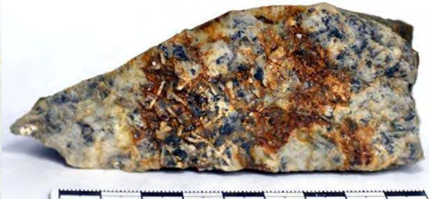
Quartz-rich veins composed largely of quartz, fluorite, cassiterite, and sulfides hosted by Catavi Fm. quartzites. Quartz is milky and massive. Fairly abundant fluorite euhedral cubic, translucent crystals (<5mm) overgrow quartz. Cassiterite crystals are dark brown in color and mm-sized. Sulfide minerals (pyrite and sphalerite?) also occur in the vein and are largely oxidized.
