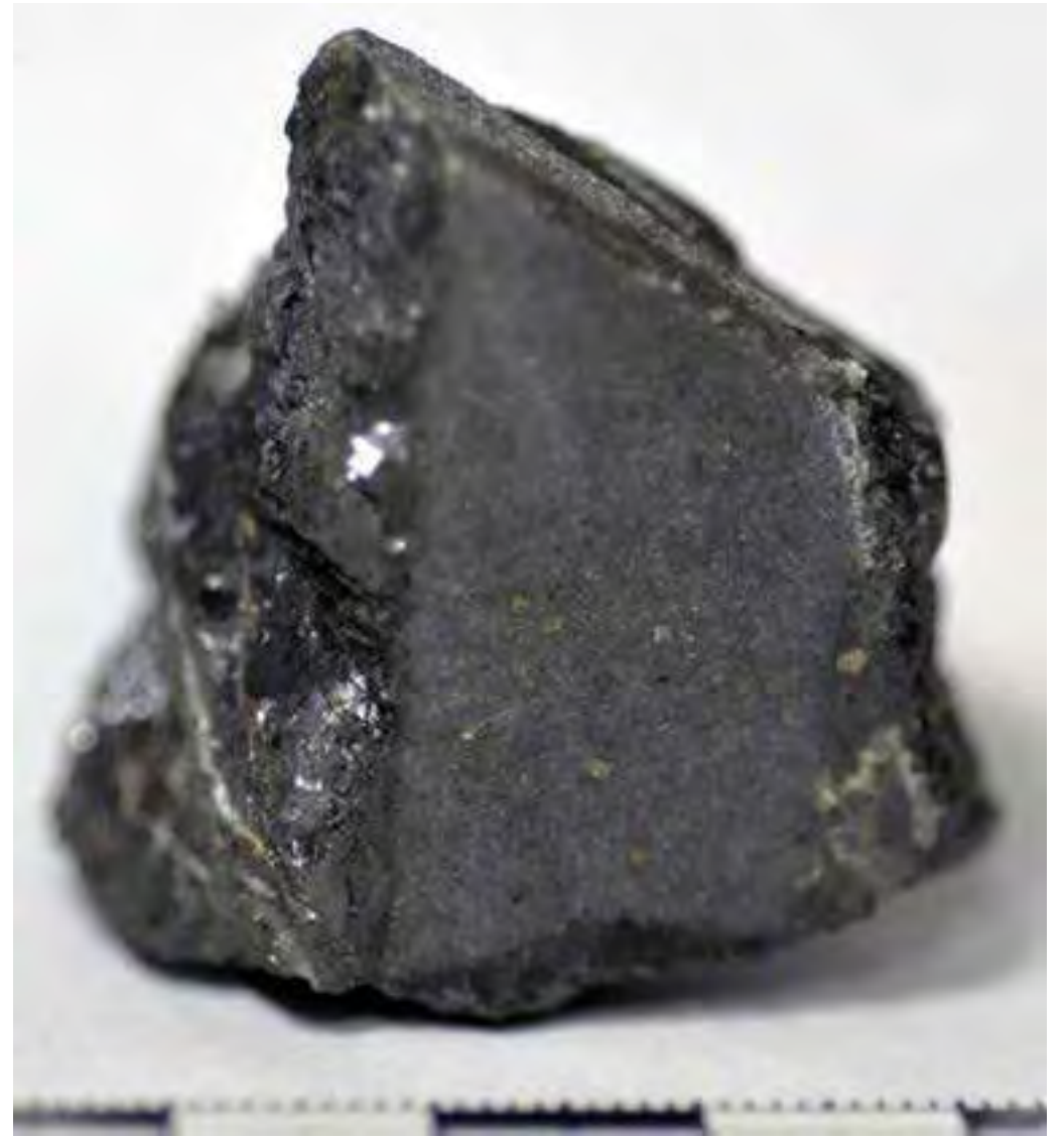
Mineralized vein composed of sphalerite, pyrite, milky massive quartz, and siderite. Sphalerite is massive and dark grey-black in color ( var. marmatite ). Pyrite forms millimetric- centimetric aggregates of subhedral-euhedral millimetric crystals and is intergrown with mm-sized subhedral platy siderite crystals. Veinlets of siderite-pyrite cut across sphalerite and milky quartz.
