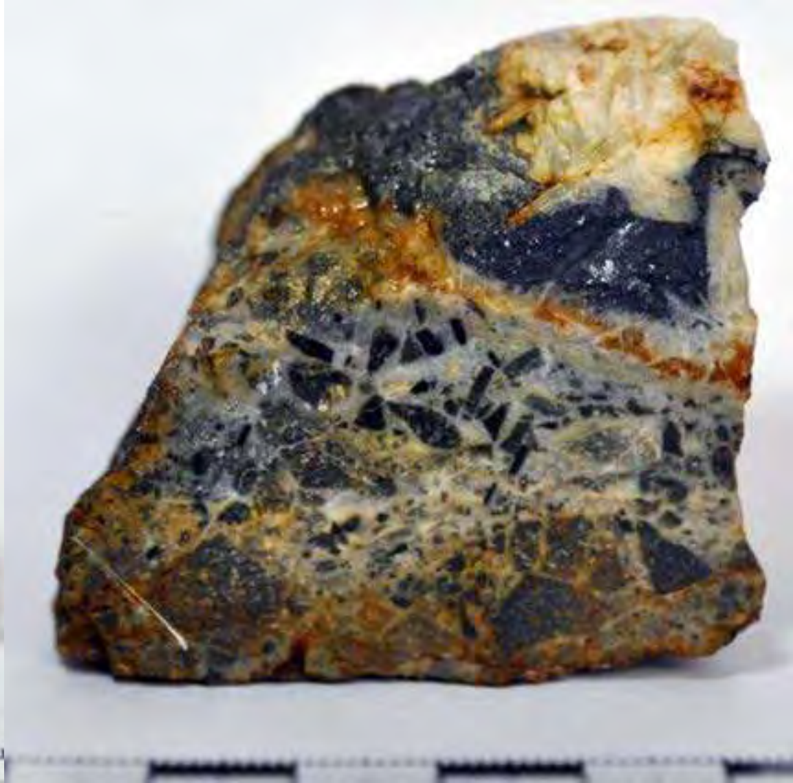
Mineralized hydrothermal breccia. Angular to sub-angular rock clasts up to 1 cm long, presumably from the hosting Catavi Fm., are cemented by semi-massive milky quartz. Some rock clasts have a porphyritic texture with white phenocrysts (<1mm), probably quartz or feldspars. The breccia is cut by a quartz-galena vein. Vein quartz crystals (1mm) are subhedral and translucent.
