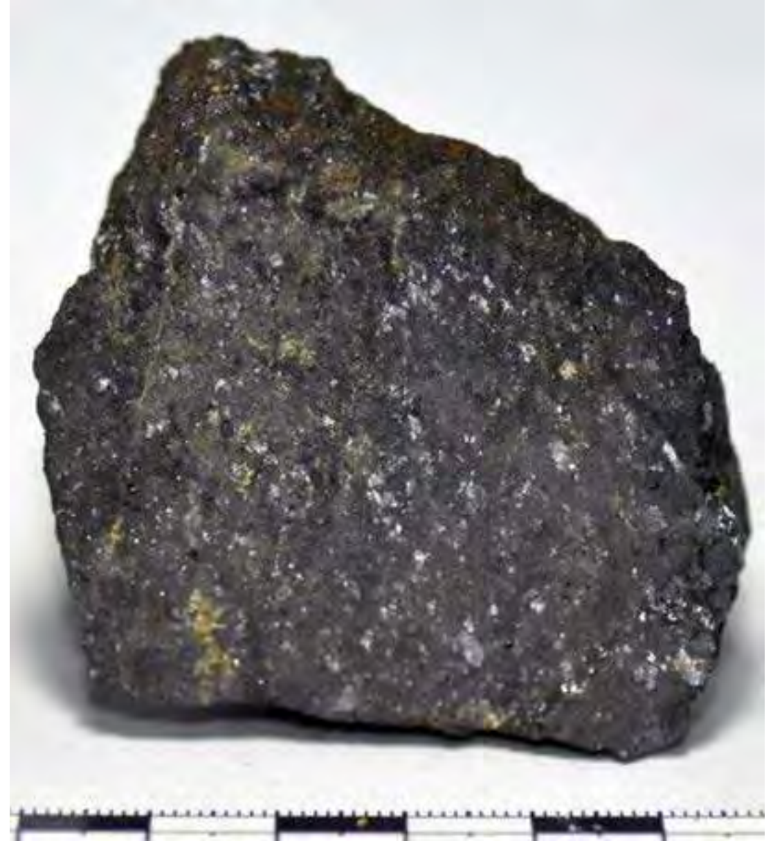
Black massive sphalerite ( var. marmatite) with lesser proportions of pyrite \pm chalcopyrite. The sample is composed in its great majority by black massive sphalerite although individual sphalerite subhedral millimetric grains are also observed. Subhedral-anhedral pyrite \pm chalcopyrite crystals appear forming mm-sized aggregates or thin veinlets across the sphalerite.
