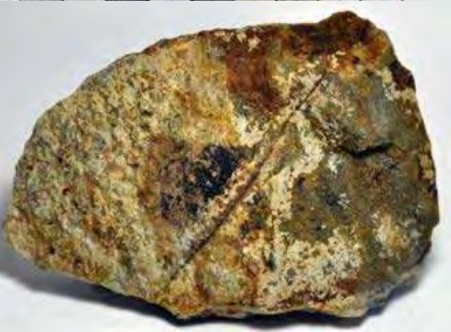
Quartz-rich veins composed largely of quartz, fluorite, cassiterite, and sulfides hosted by Catavi Fm. quartzites. Quartz is milky and massive. Fairly abundant fluorite euhedral cubic, translucent crystals (<5mm) overgrow quartz. Cassiterite crystals are dark brown in color and mm-sized. Sulfide minerals (pyrite and sphalerite?) also occur in the vein and are largely oxidized.
