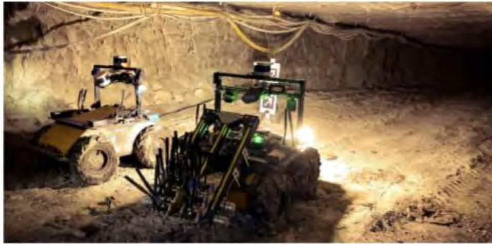
Figura D.4: Two autonomous ground rovers (Husky A200) explore the network of underground tunnels at the Arch mines.
