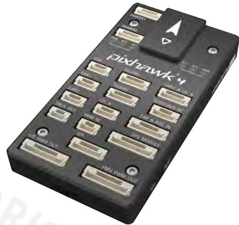
Pixhawk<sup>®</sup> 4 is the latest update to the successful family of Pixhawk flight controllers. It was designed and developed in collaboration with Holybro and the PX4 team, optimized to run the full Dronecode stack, and comes pre-installed with the latest PX4 firmware.
