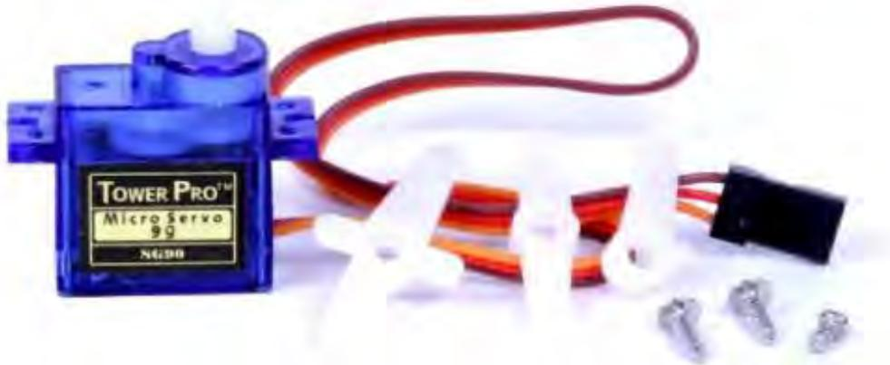
Tiny and lightweight with high output power. Servo can rotate approximately 180 degrees (90 in each direction), and works just like the standard kinds but smaller. You can use any servo code, hardware or library to control these servos. Good for beginners who want to make stuff move without building a motor controller with feedback & gear box, especially since it will fit in small places. It comes with a 3 horns (arms) and hardware.
