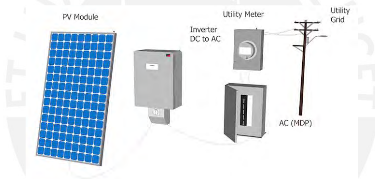
Figure 7: Grid-connected PV system.
