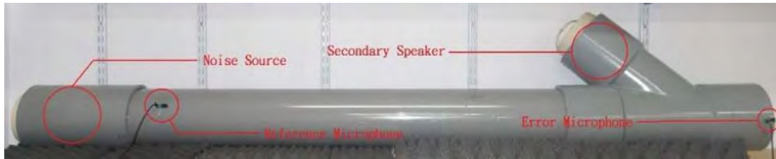
Figure 2.10: Duct system (Chen, et al., 2017)
