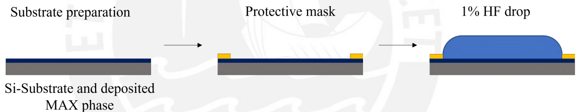
Figure 2.20 Etching process with 1% HF by using a Teflon protective mask (indicated in yellow)
