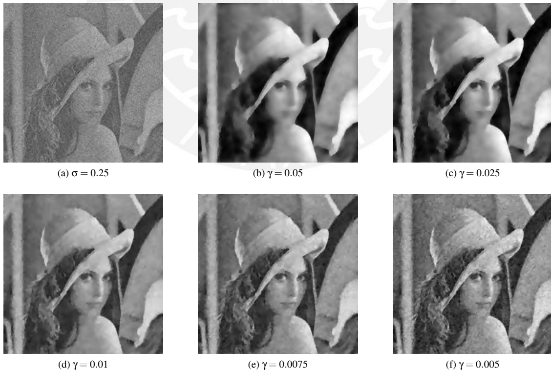
Figure A.2: Reconstructed images from a noisy greyscale Lena with \sigma = 0.25 for additive Gaussian noise using Ql_0 -grad and different values of \gamma .
