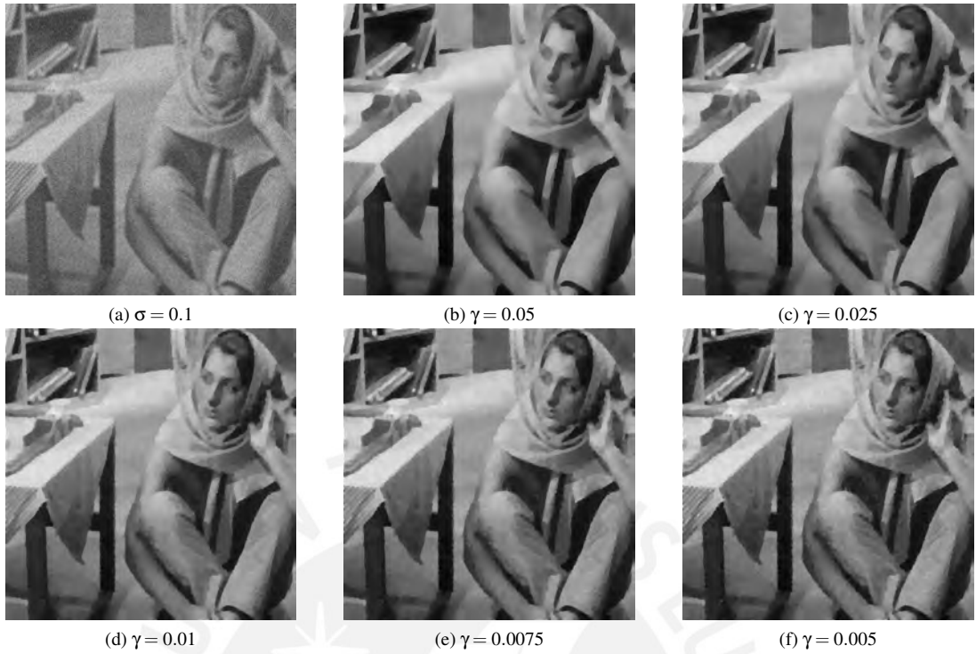
Figure 4.54: Reconstructed images from a noisy greyscale Barbara with \sigma = 0.1 for additive Gaussian noise and an average 5 \times 5 filter, using Q\ell_0 -grad and different values of \gamma .
