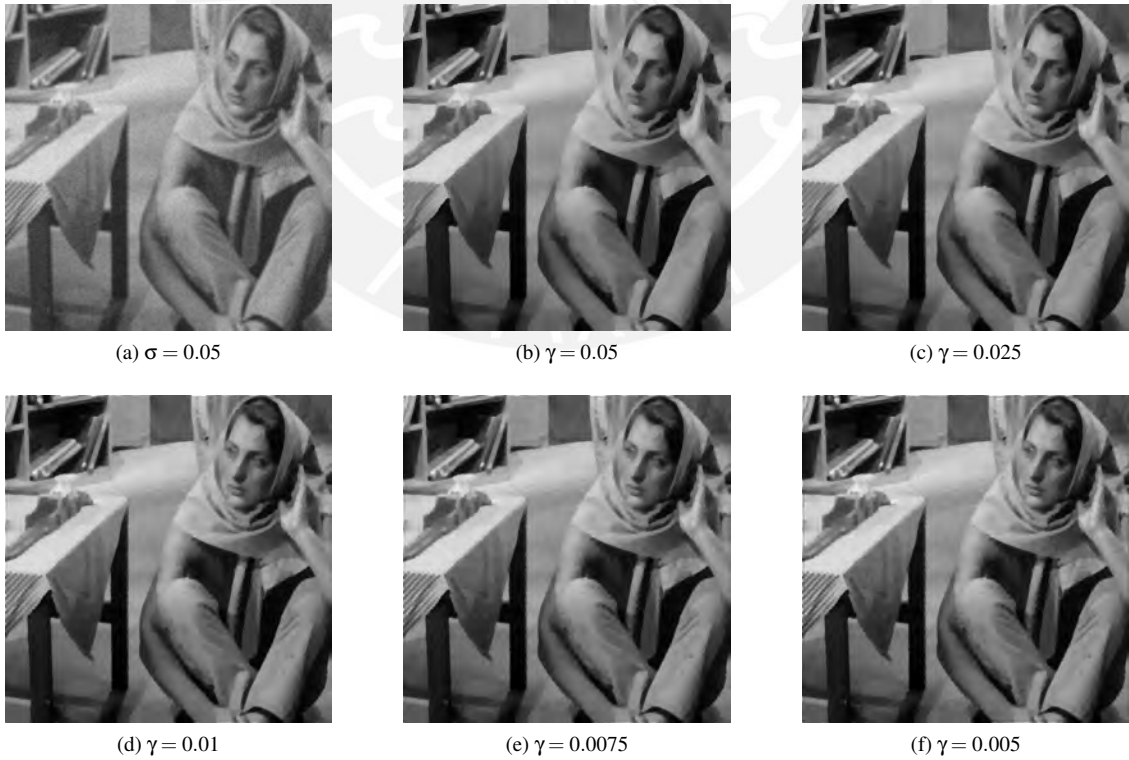
Figure A.5: Reconstructed images from a noisy greyscale Barbara with \sigma = 0.05 for additive Gaussian noise and an average 5 \times 5 filter, using Q\ell_0 -grad and different values of \gamma .
