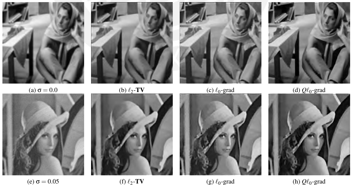
Figure 4.31: Reconstructed images with l_2 -TV, l_0 -grad and Ql_0 -grad from a noisy image with different \sigma for additive Gaussian noise and a Gaussian 9 \times 9 filter.
