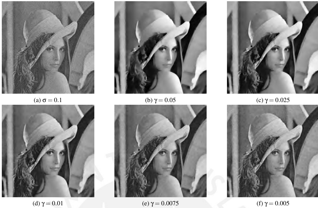
Figure 4.52: Reconstructed images from a noisy greyscale Lena with \sigma = 0.1 for additive Gaussian noise using Ql_0 -grad and different values of \gamma .
