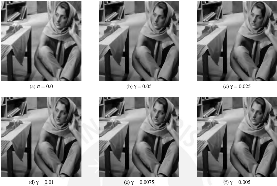
Figure A.4: Reconstructed images from a noisy greyscale Barbara with \sigma = 0.0 for additive Gaussian noise and an average 5 \times 5 filter, using Q\ell_0 -grad and different values of \gamma .
