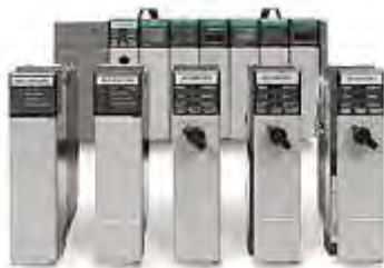
Figura A.13. PLC Allen Bradley SLC-500 (Rockwell Automation, 2019)
