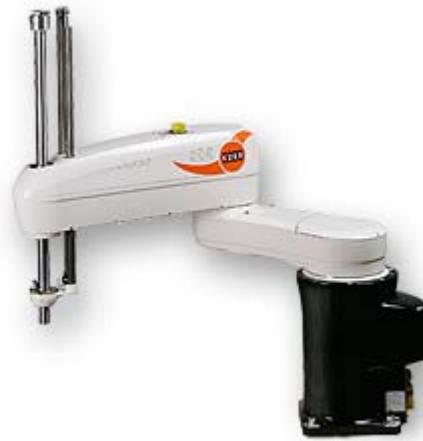
Figura 3. Robot SCARA KR 10 scara R850 [4]
