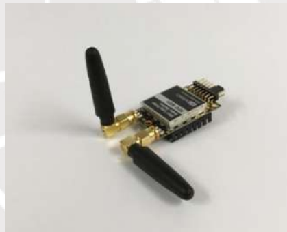
Figure 8-1: Antenna configuration to achieve polarisation diversity
