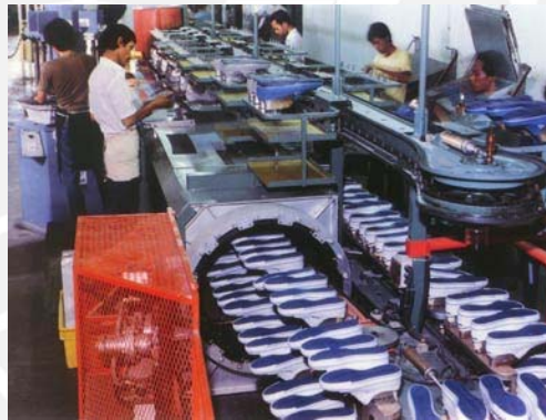
Fig. 2.2 Carga automática de autoclaves (Anzani spa-Vulcomatic, Machines for footwear, leather goods, garments)
