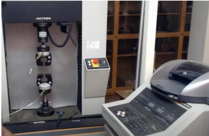
Figura 4.14. Equipo usado en el ensayo ASTM D6693 “Standard Test Method for Determining Tensile Properties of Nonreinforced Polyethylene and Nonreinforced Flexible Polypropylene Geomembranes,”.
