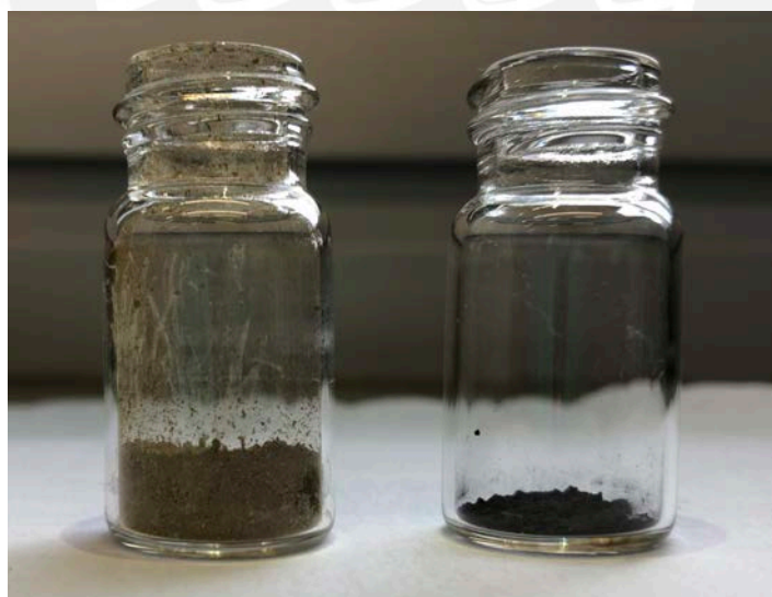
Figure 4-2. Image of 100 mg Si nanopowder (left) and porous Si nanopowder (right) in a 5 mL vial
