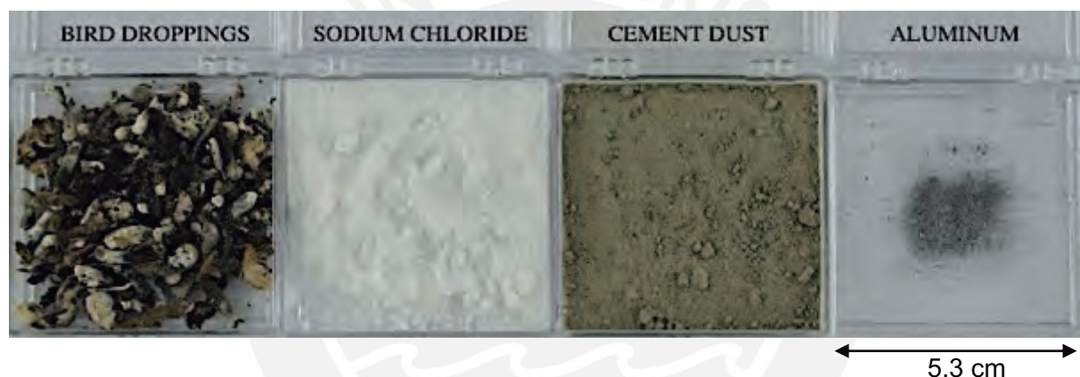
Figure 11. Four types of contaminants applied to the glass surface before artificial and natural weathering.
