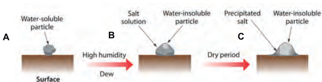
Figure 6. Cementation process [72]. A) Deposition of an inorganic particle that contains water-soluble and insoluble salts. B) Formation of salt solution retaining insoluble particles at high humidity. C) Formation of precipitated salt, keeping the insoluble particle attached to the glass surface after drying.
