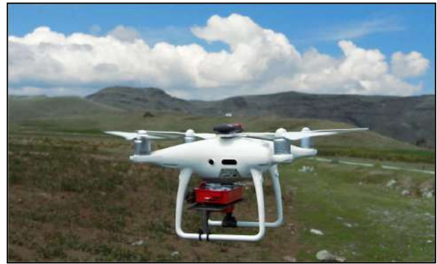
Fig. 4. DJI Phantom 4 with onboard Micasense Rededge Camera.
