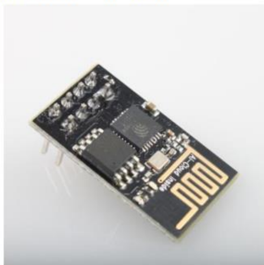
Figure 3 [Module Pin Counts, 8 pin, 14.3 mm *24.8 mm *3.0 mm]
