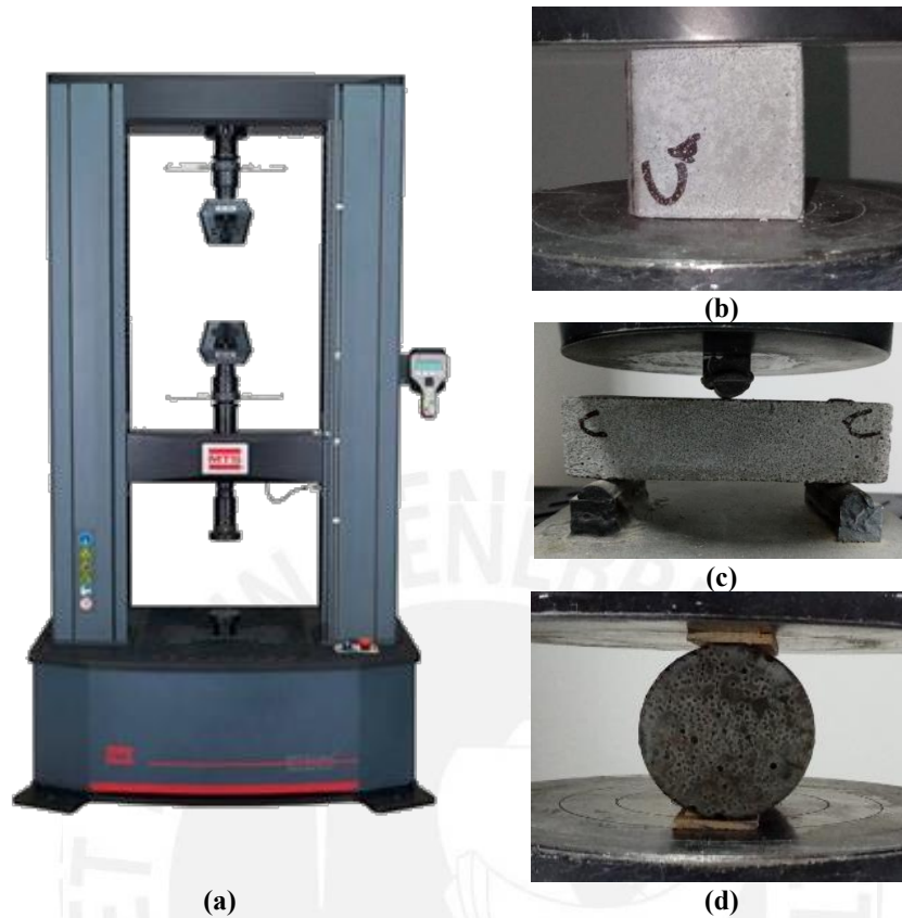
Figure 5.5 Mechanical test for the fly ash-based geopolymers: (a) electromechanical machine (Exceed E45, MTS, USA) (Direct Industry, n.d.-b), (b) specimens for compressive strength, (c) specimens for flexural strength, and (d) specimens for splitting tensile strength test.
