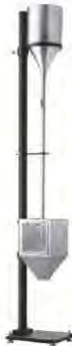
FIG. 1 Apparatus for Falling Sand Abrasion Test
