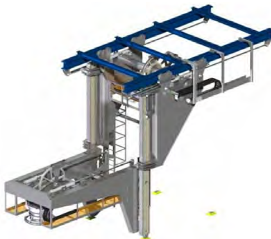
Figura 2.8: LARS tipo ORS. (Sepro Technology, s.f)
