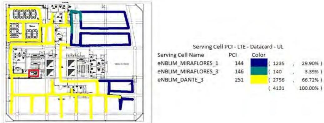
Figura 29: Traza Serving Cell PCI UL.
