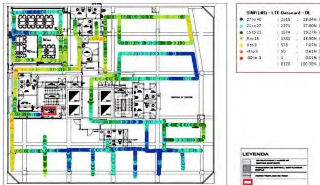
Figura 37: Trazo SINR DL SMALL CELL ON.
