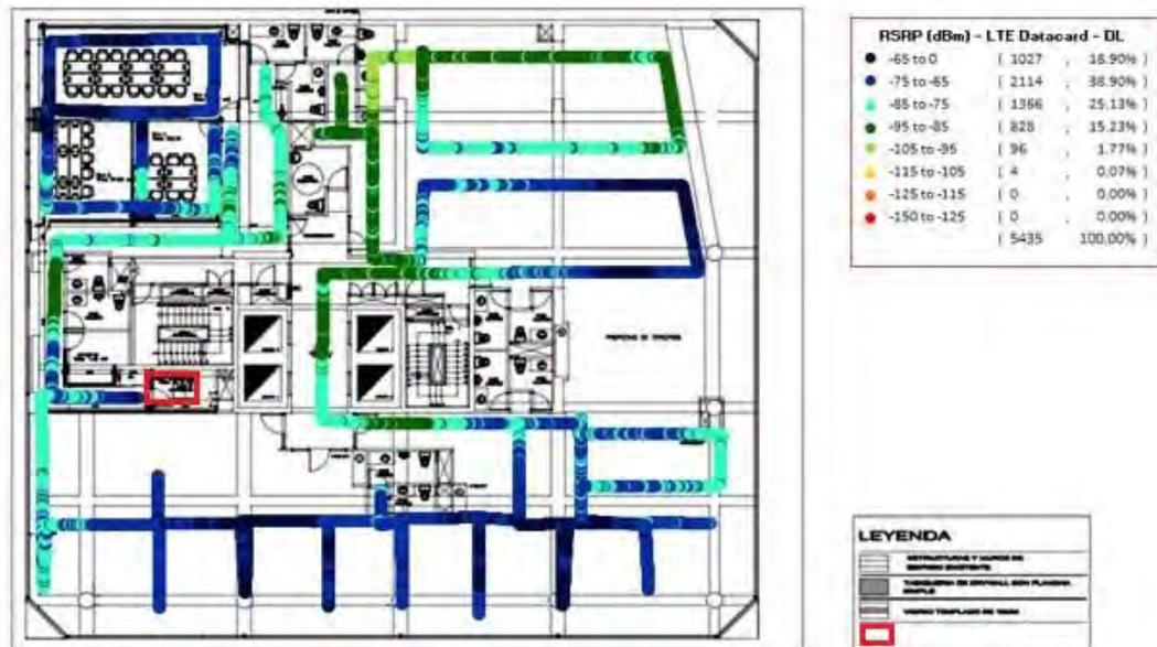
Figura 35: Traza RSRP DL SMALL CELL ON.
