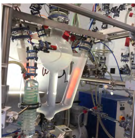
Figure 4.14: Picture of the Reboiler
