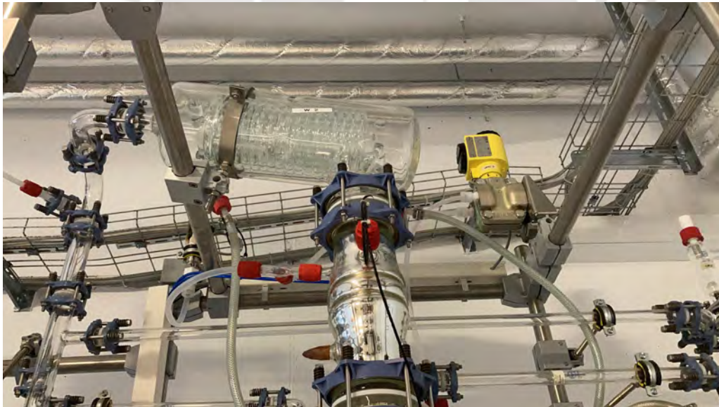
Figure 4.10: Picture of the Condenser
