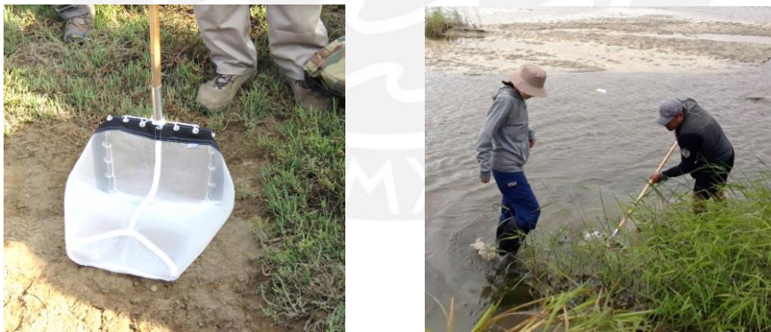
Figure 4.7 Sampling process using a kick net of 300\ \mu\text{m} mesh
