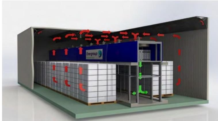
Figura 1.18: Túnel de Pre-frio (Energroup 2016)
