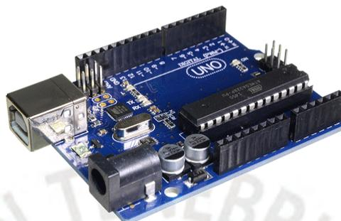
Fig 2.17 Micro controlador Arduino Uno R3
