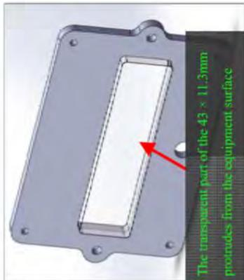
3. The intermediate part of 43\*11.3mm is the protuberant transparent window, when it is installed on the panel of the equipment, cut out the opening according to this size, and expose the transparent display window.
