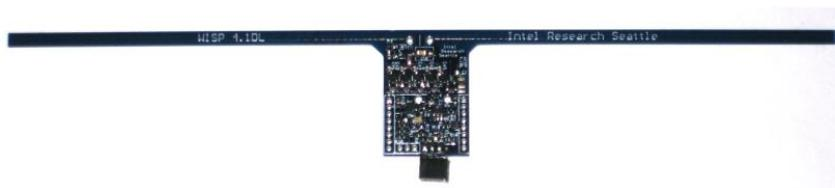
Fig. 2.1: Etiqueta RFID UHF: WISP 5 [16]
