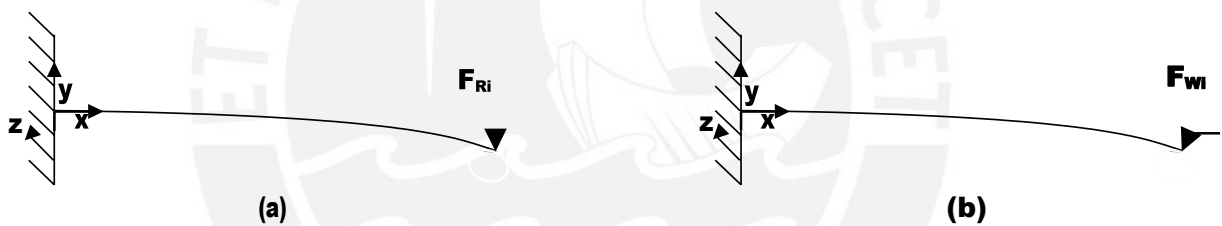
Figure 5.8: Clamped bending beam with force imprint at the end of the beam:
