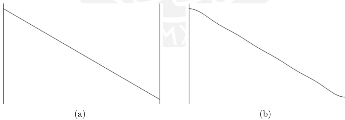
Figure 2.4: Comparison between (a) eq. 2.21 and (b) eq. 2.14 with n = 8 for Couette flow considering eq. 2.23
