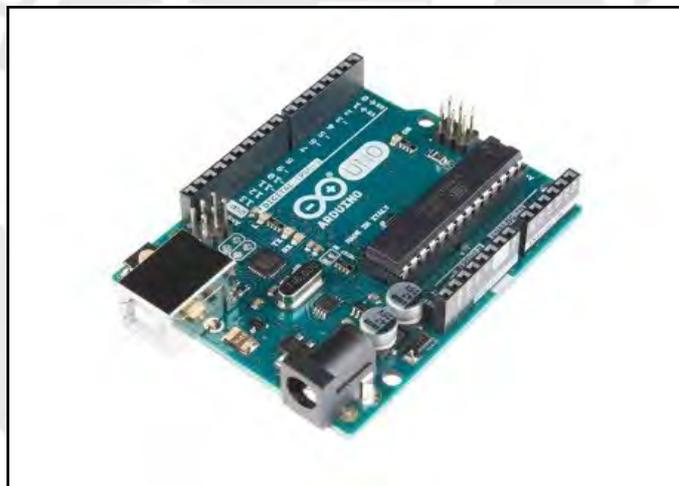
**Figura 60.** Arduino UNO Rev.3
