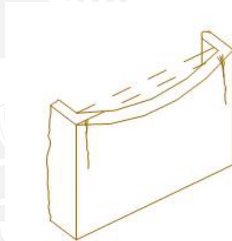
Damage on corners by Traction – flectional strength (photograph by San Bartolomé 2002)
