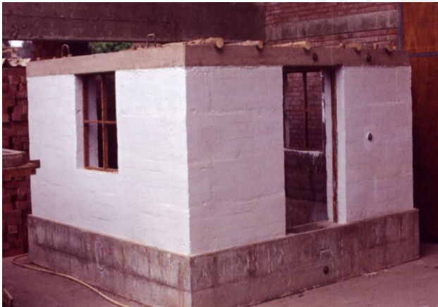
New construction with canes and concrete beam before seismic test (left) and after seismic test (right) (photograph by San Bartolomé 2002)
