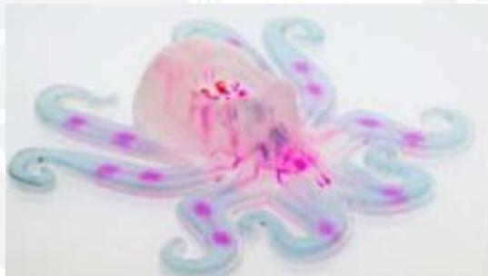
Figura 1.11: Robot flexible *Octobot* [Laschi , 2016]
